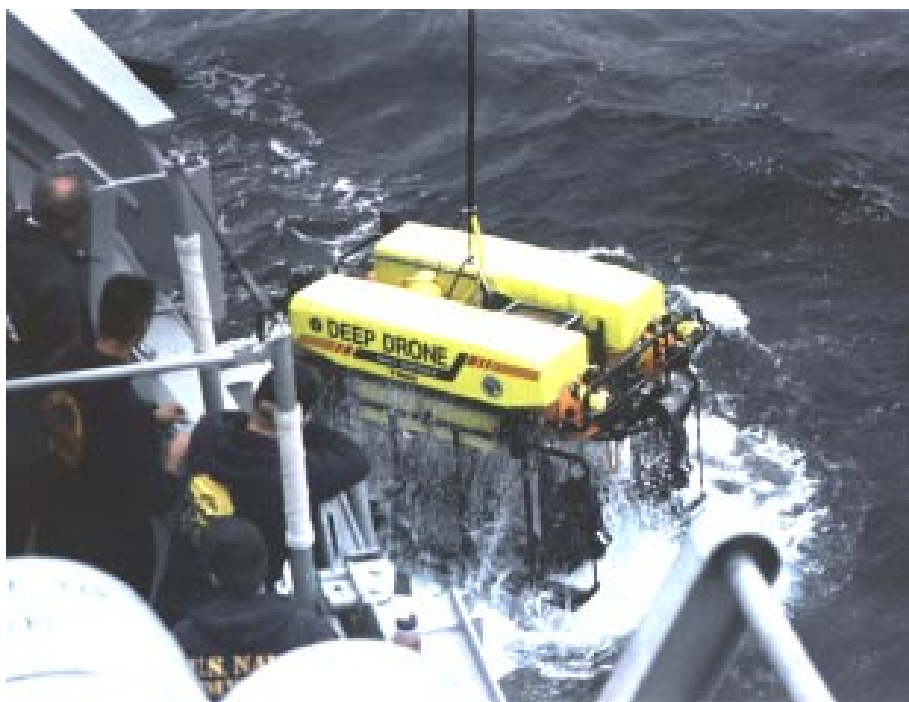
Deep Drone 7200 returns to the USS Grapple due to extremely heavy seas. Deep Drone was used to help Grapple's divers locate victims and wreckage. (Navy photograph by Photographer's Mate Airman Charles L. Withrow.)
